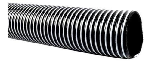
**Freeze-resistant slurry tanker suction and discharge hose with a rigid PVC spiral**. A special material blend ensures that the hose remains flexible even at very low external temperatures. It is resistant to cracking during bending tests and has strong mechanical properties. Suitable for use in municipal vehicles, tank trucks, and as a pipeline component. The hose is used for transferring fluids such as slurry, dirty water, light water-based chemicals, or fecal matter.
