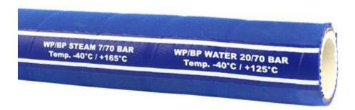
Low-pressure hose for steam and water, certified and approved for food contact. Designed for use in the food industry, it is resistant to UV radiation, ozone, and atmospheric conditions. The outer hose construction is micro-perforated to prevent the "popcorning" effect. This hose can also be used for transporting hot water up to +125°C and glycol. It is compatible with all water and steam coupling systems (do not crimp the steam hose hydraulically).
