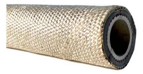
A highly durable industrial hose with a glass fiber jacket and an EPDM layer. It is used in foundries, steel mills, and maritime vessels to transfer coolant (hot water, glycol) in environments with very high temperatures, such as installations near smelting furnaces. The hose remains electrically non-conductive, and its insulation is resistant to minor splashes of molten metal or sparks.
