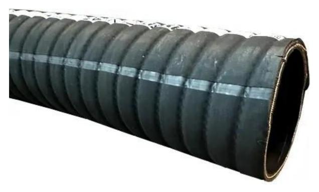
**Strong and flexible rubber suction/discharge (S/D) hose**, reinforced with two textile plies and a double steel spiral.
