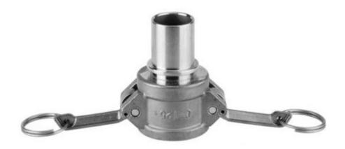
Female CAMLOCK coupling type CS with a smooth hosetail designed for secure attachment using shell clamps. Manufactured according to the US standard MIL-C-27847 (A-A-59326). This is one of the most widely used quick coupling systems in industrial applications across Europe.
