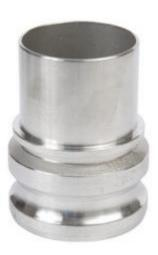
Male CAMLOCK coupling type ES with a smooth hosetail attached only to shell clamps. Manufactured according to the US standard MIL-C-27847 (A-A-59326). This is one of the most widely used quick coupling systems in industrial applications across Europe.
