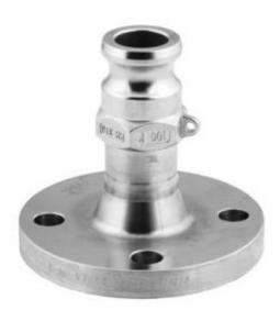
Male CAMLOCK coupling type FLA, ended by fixed flange PN10/16, EN 1092-02/04 norm, and manufactured according to the US standard MIL-C-27847 (A-A-59326). This is one of the most widely used quick coupling systems in industrial applications across Europe.
