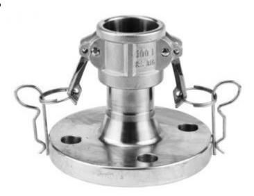
Female CAMLOCK coupling type FLB with NBR gasket, ended by fixed flange PN10/16, EN 1092-02/04 norm, and manufactured according to the US standard MIL-C-27847 (A-A-59326). This is one of the most widely used quick coupling systems in industrial applications across Europe.
