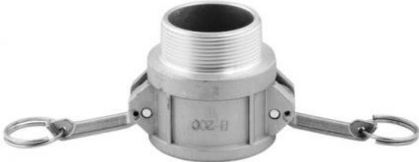
**Female CAMLOCK coupling type B with external BSP thread.** Manufactured according to the US standard MIL-C-27847 (A-A-59326). This is one of the most widely used quick coupling systems in industrial applications across Europe.
