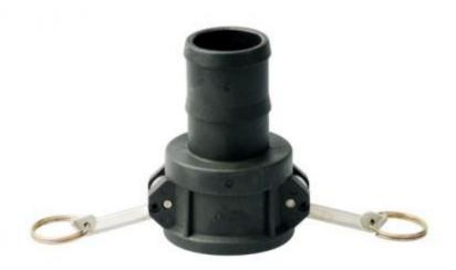
**Female CAMLOCK coupling type C with ribbed hosetail**. Manufactured according to the US standard MIL-C-27847 (A-A-59326). This is one of the most widely used quick coupling systems in industrial applications across Europe.
