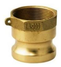
Male CAMLOCK coupling type A with internal BSP thread. Manufactured according to the US standard MIL-C-27847 (A-A-59326). This is one of the most widely used quick coupling systems in industrial applications across Europe.
