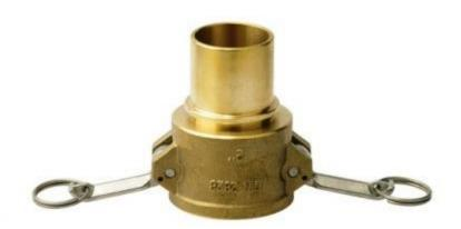
Female CAMLOCK coupling type CS with a smooth hosetail designed for secure attachment using shell clamps. Manufactured according to the US standard MIL-C-27847 (A-A-59326). This is one of the most widely used quick coupling systems in industrial applications across Europe.
