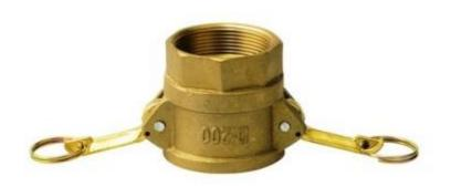
**Female CAMLOCK coupling type D with internal BSP thread**. Manufactured according to the US standard MIL-C-27847 (A-A-59326). This is one of the most widely used quick coupling systems in industrial applications across Europe.
