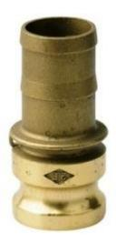
Male CAMLOCK coupling type ES with a smooth hosetail attached only to shell clamps, and manufactured according to the US standard MIL-C-27847 (A-A-59326). This is one of the most widely used quick coupling systems in industrial applications across Europe.
