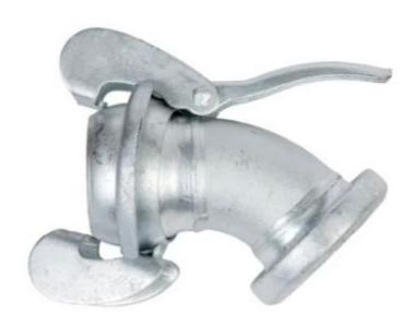
The BAUER-BELOK quick coupler type S12/B12 with 45° bend. The fitting construction consists of a male BAUER part with lever x female BAUER part with SBR O-Ring.
